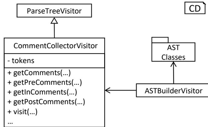
Figure 3.8: The *CommentCollectorVisitor*: The visitor implements a process for the collection of comments in arbitrary nodes of the parse tree. In order to simplify the processing, merely the *visit* method has to be called. This method delegates the work to the *getComments* function and finally returns all collected comments. The comment collector extends the *ParseTreeVisitor* and is called within the *ASTBuilderVisitor* whenever an AST is constructed.
