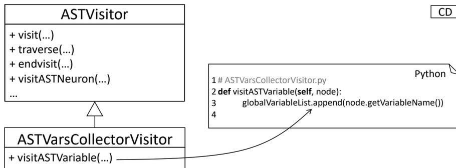
Figure 3.25: The *visitor* pattern in practice [KRV10]: Even small operations, e.g., the collection of certain types of variables, require the usage of sub-classing, where only a single operation is redefined.
