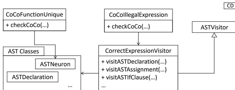
Figure 3.20: Simple and complex context conditions: Simple context conditions such as *CoCoFunctionUnique* can be implemented in a single function, while more complex conditions such as *CoCollegalExpression* also utilize additional classes and visitors. Both types of context conditions work on the handed over AST.
