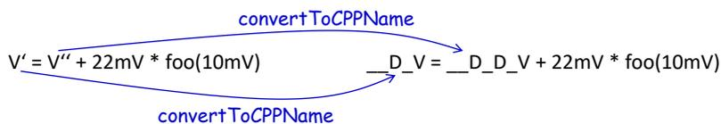
Figure 4.13: Adaption of syntax by the *convertToCPPName* method.
