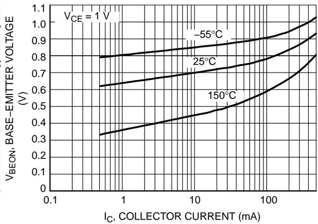
Figure 4. Base-Emitter Voltage
