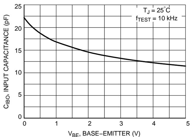
Figure 6. Input Capacitance
