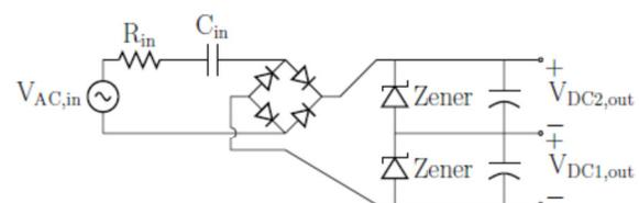
Transformerless Supply with Dual Output Zeners
