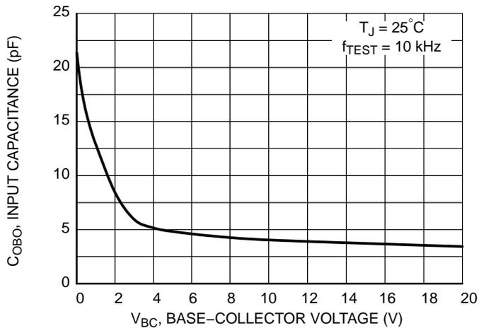
Figure 7. Output Capacitance
