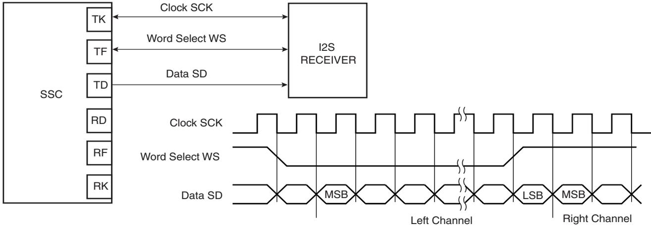
**Figure 33-18.** Codec Application Block Diagram
