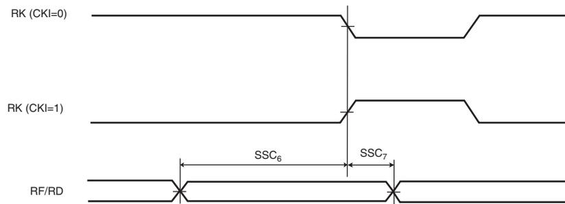
**Figure 41-17. SSC Receiver, RK in input and RF in Output**
