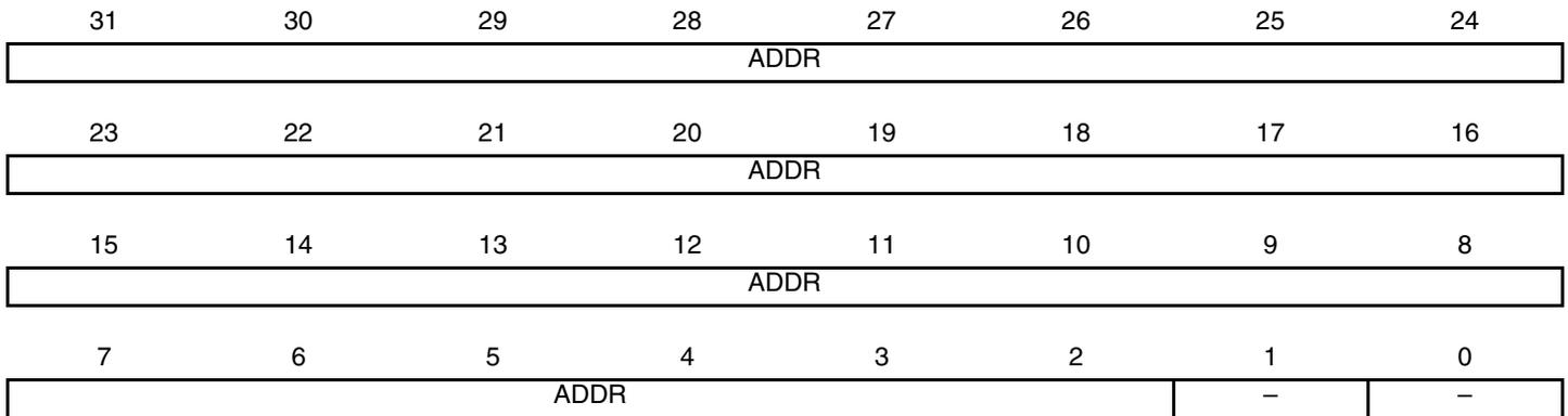
This register points to the entry in the receive buffer queue (descriptor list) currently being used. It is written with the start location of the receive buffer descriptor list. The lower order bits increment as buffers are used up and wrap to their original values after either 1024 buffers or when the wrap bit of the entry is set.
