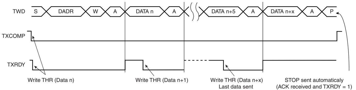
**Figure 31-8. Master Write with One Byte Internal Address and Multiple Data Bytes**
