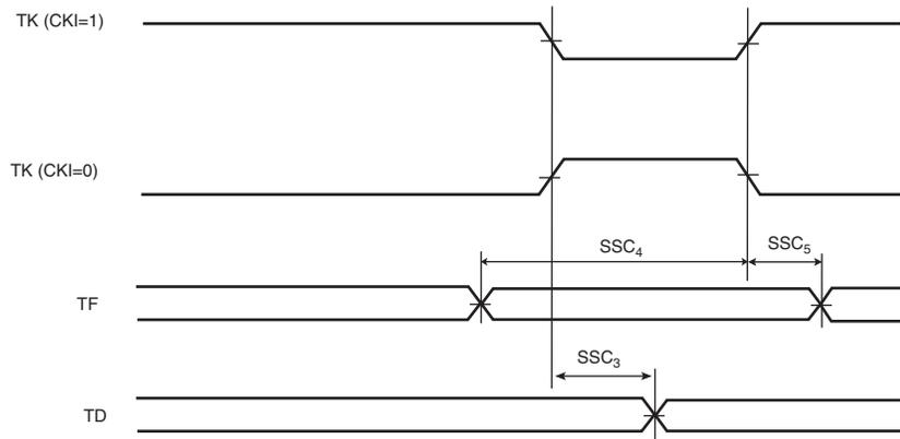
**Figure 41-16. SSC Receiver RK and RF in Input**
