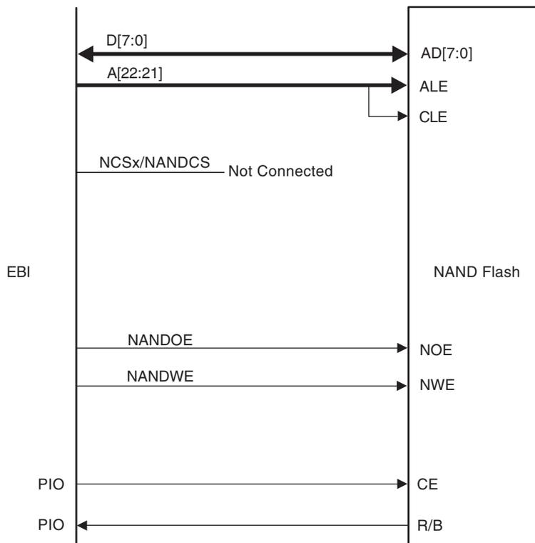
Note: The External Bus Interface is also able to support 16-bit devices.
