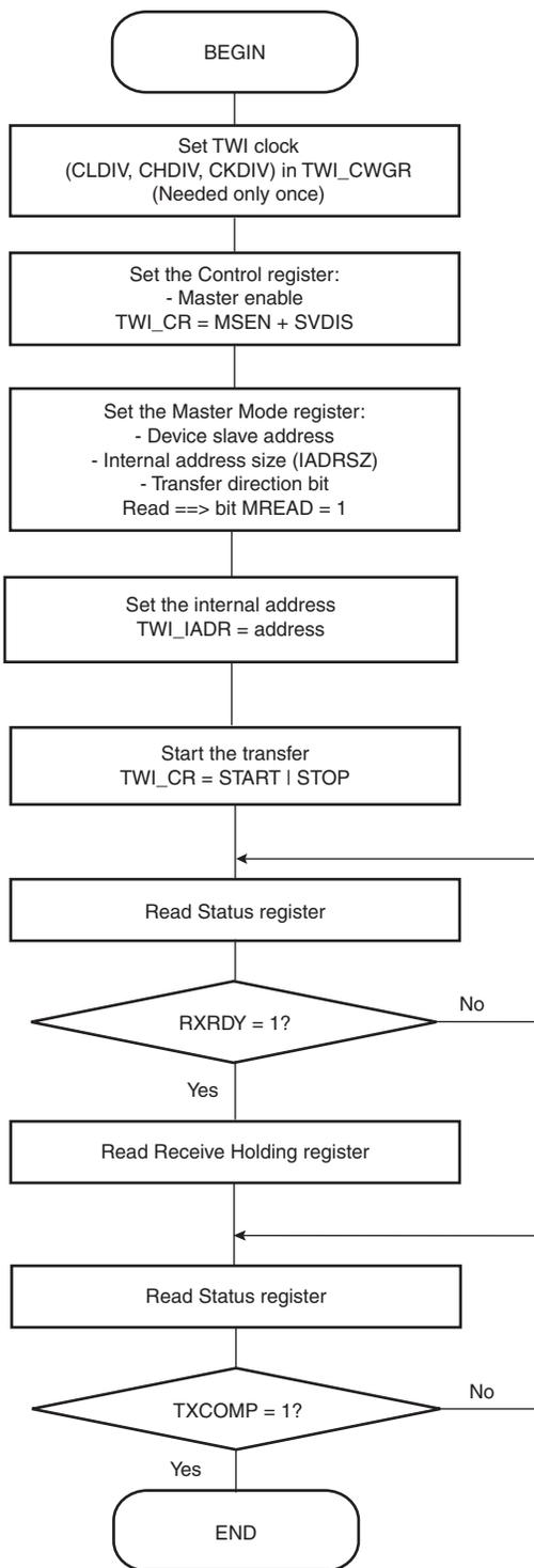
**Figure 31-19.** TWI Read Operation with Multiple Data Bytes with or without Internal Address
