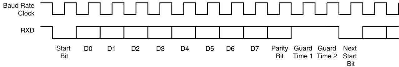
**Figure 32-32.** T = 0 Protocol with Parity Error
