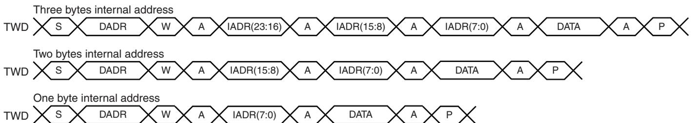
**Figure 31-12.** Master Read with One, Two or Three Bytes Internal Address and One Data Byte
