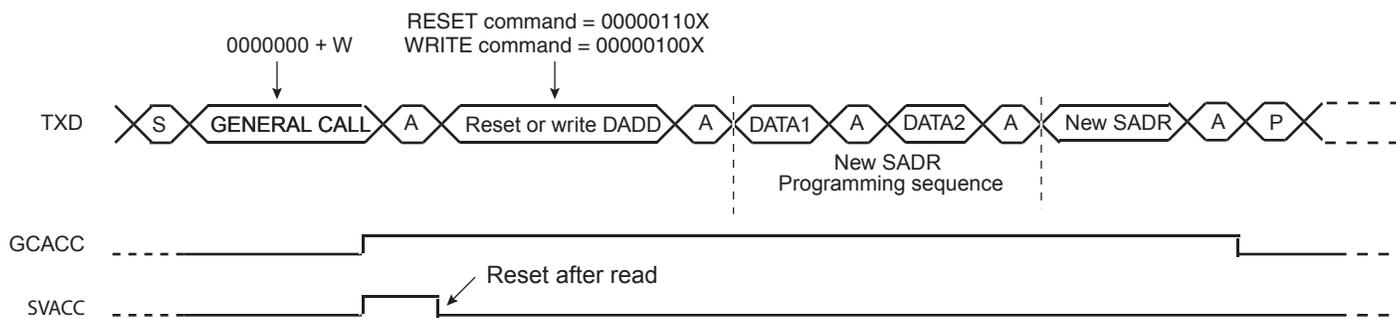
Note: This method allows the user to create an own programming sequence by choosing the programming bytes and the number of them. The programming sequence has to be provided to the master.
