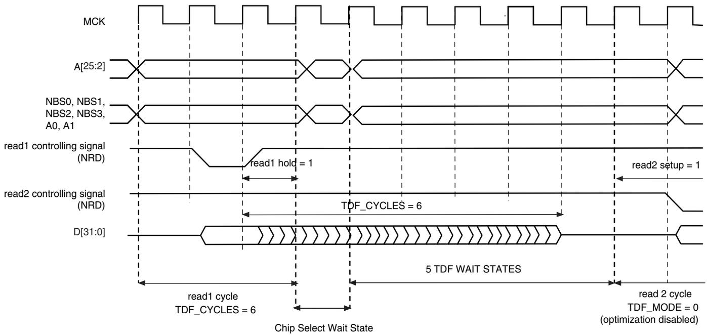
**Figure 21-25.** TDF Mode = 0: TDF wait states between a read and a write access on different chip selects
