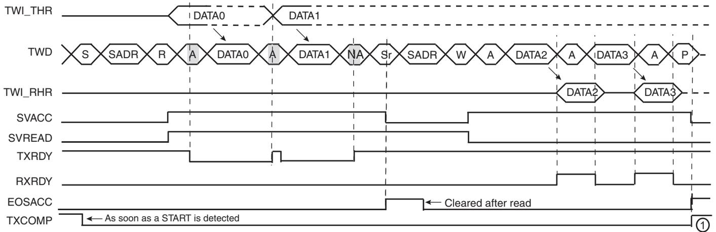
1. TXCOMP is only set at the end of the transmission because after the repeated start, SADR is detected again.
