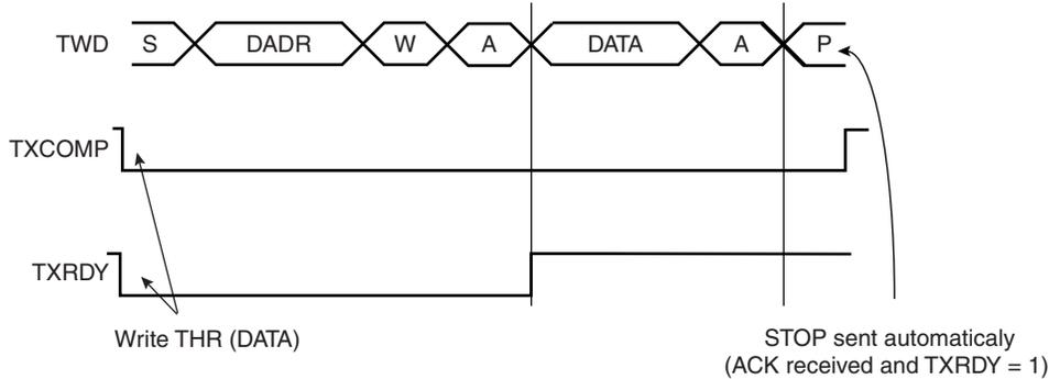
**Figure 31-7. Master Write with Multiple Data Byte**
