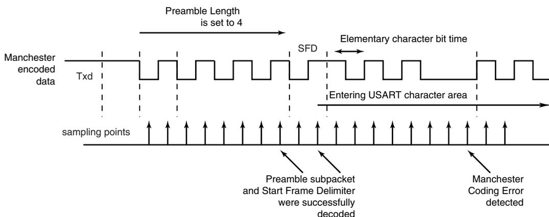
When the start frame delimiter is a sync pattern (ONEBIT field at 0), both command and data delimiter are supported. If a valid sync is detected, the received character is written as RXCHR field in the US\_RHR register and the RXSYNH is updated. RXCHR is set to 1 when the received character is a command, and it is set to 0 if the received character is a data. This mechanism alleviates and simplifies the direct memory access as the character contains its own sync field in the same register.
