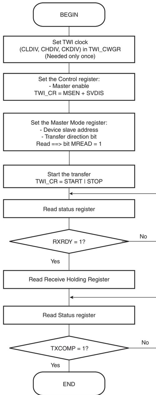
**Figure 31-18.** TWI Read Operation with Single Data Byte and Internal Address
