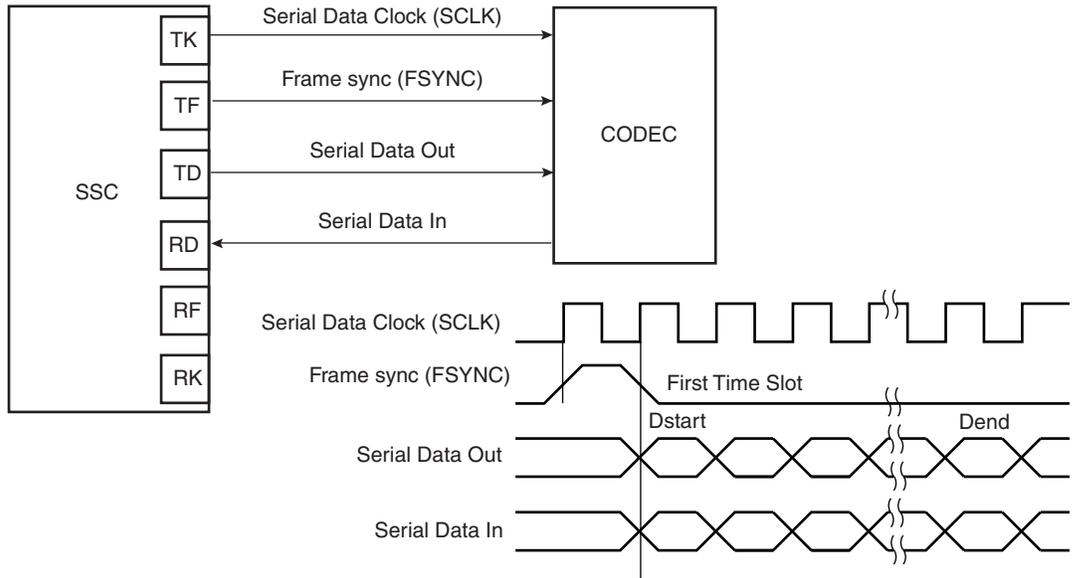
**Figure 33-19. Time Slot Application Block Diagram**
