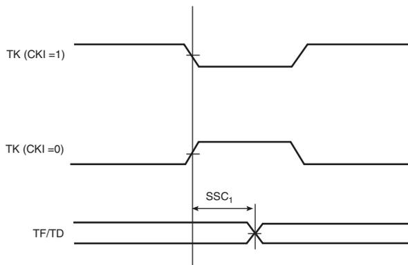
**Figure 41-14. SSC Transmitter, TK in Output and TF in Input**
