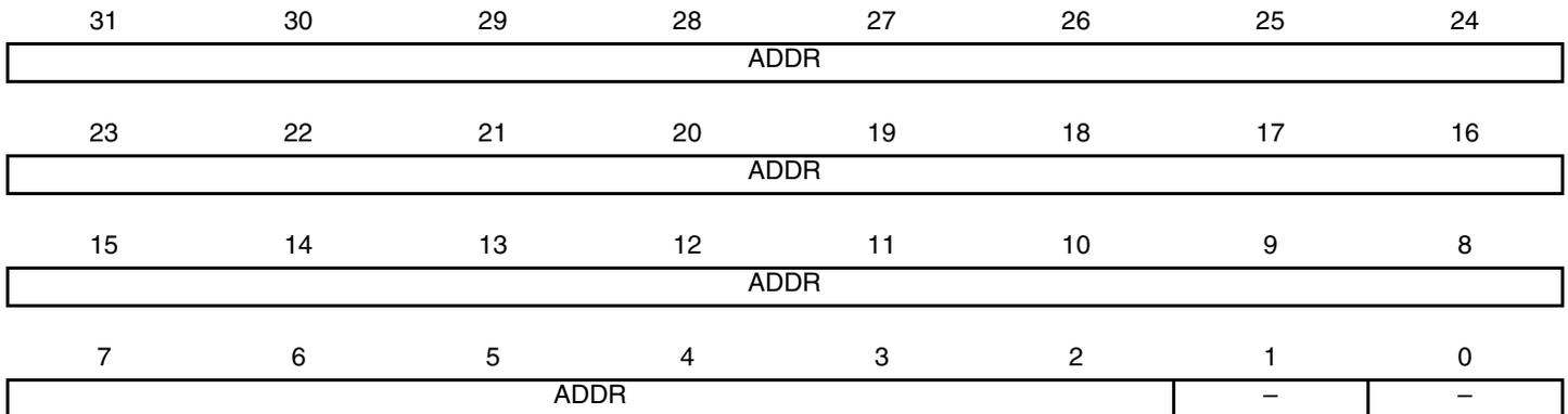
This register points to the entry in the transmit buffer queue (descriptor list) currently being used. It is written with the start location of the transmit buffer descriptor list. The lower order bits increment as buffers are used up and wrap to their original values after either 1024 buffers or when the wrap bit of the entry is set. This register can only be written when bit 3 in the transmit status register is low.
