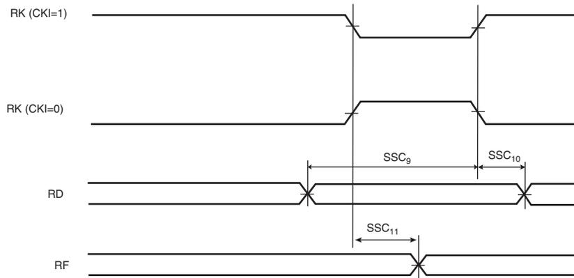
**Figure 41-19. SSC Receiver, RK in Output and RF in Input**
