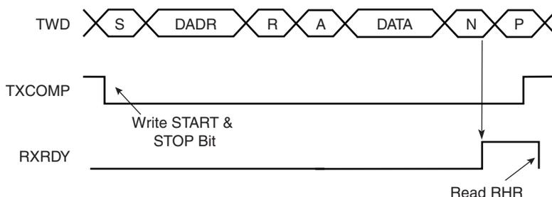
**Figure 31-10.** Master Read with Multiple Data Bytes
