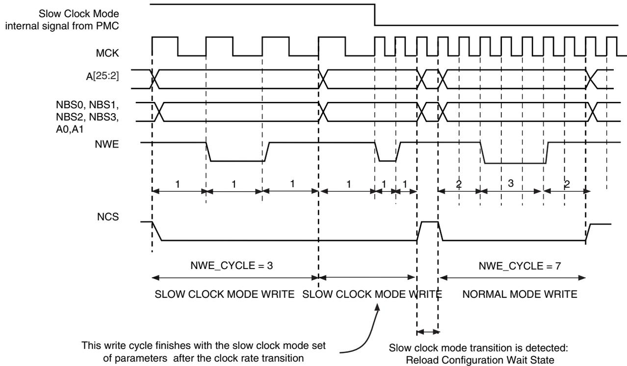
**Figure 21-34.** Recommended Procedure to Switch from Slow Clock Mode to Normal Mode or from Normal Mode to Slow Clock Mode
