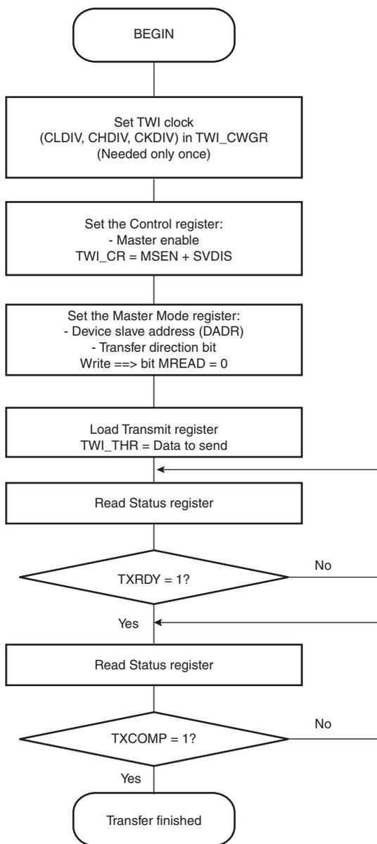
**Figure 31-15. TWI Write Operation with Single Data Byte and Internal Address**
