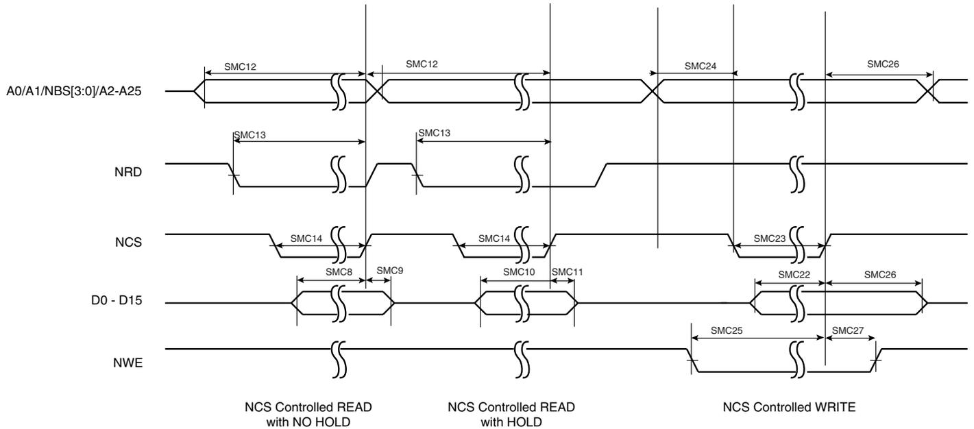
**Figure 41-4. SMC Timings - NRD Controlled Read and NWE Controlled Write**
