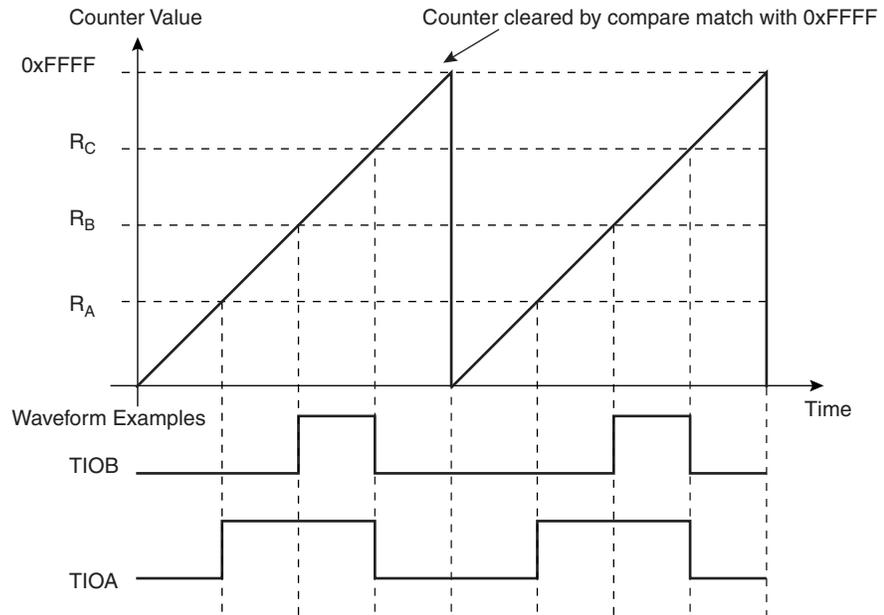
**Figure 34-8.** WAVSEL= 00 with trigger
