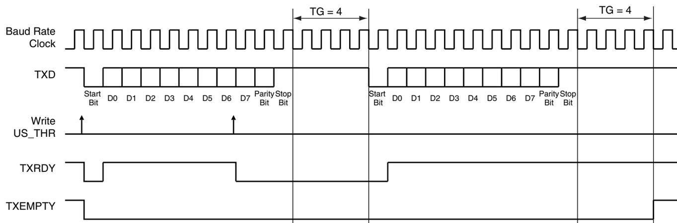
Table 32-7 indicates the maximum length of a timeguard period that the transmitter can handle in relation to the function of the Baud Rate.
