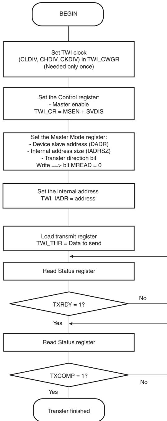
**Figure 31-16.** TWI Write Operation with Multiple Data Bytes with or without Internal Address
