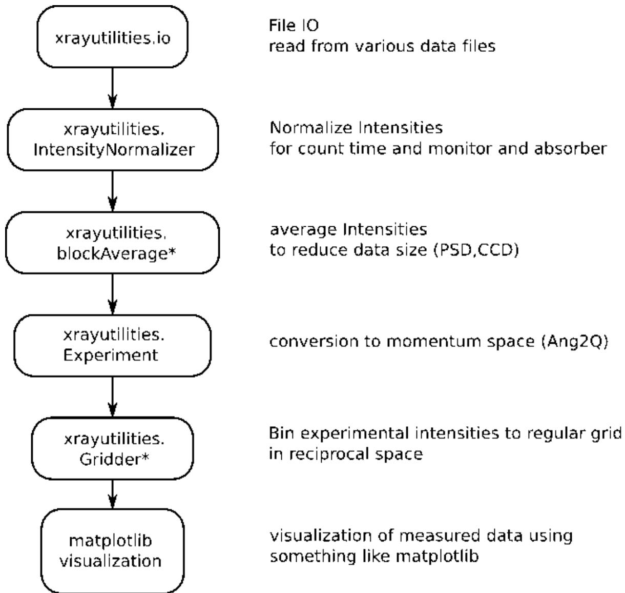
*xrayutilities* provides a set of functions to read experimental data from various data file formats. All of them are gathered in the `io`-subpackage. After reading data with a function from the `io`-submodule the data might be corrected for monitor counts and/or absorption factor of a beam attenuator. A special set of functions is provided to perform this for point, linear and area detectors.
