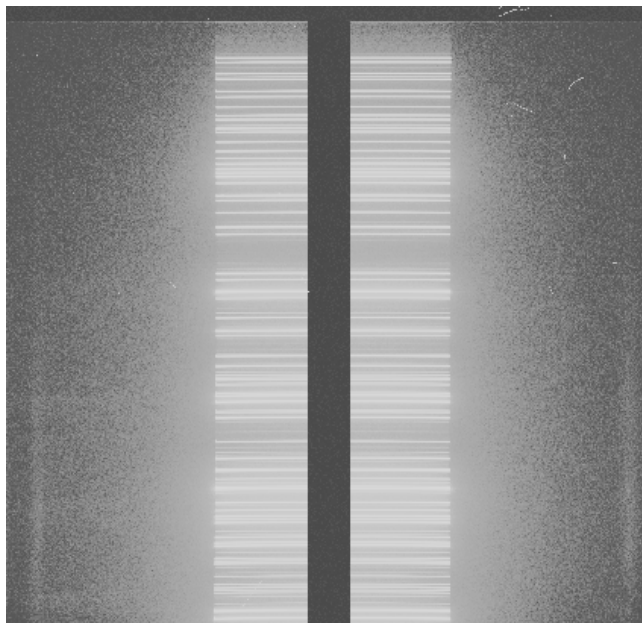
Figure 4. An arc taken with 2-amp readout (L2, U2). Note the overscans in the middle and the top.
