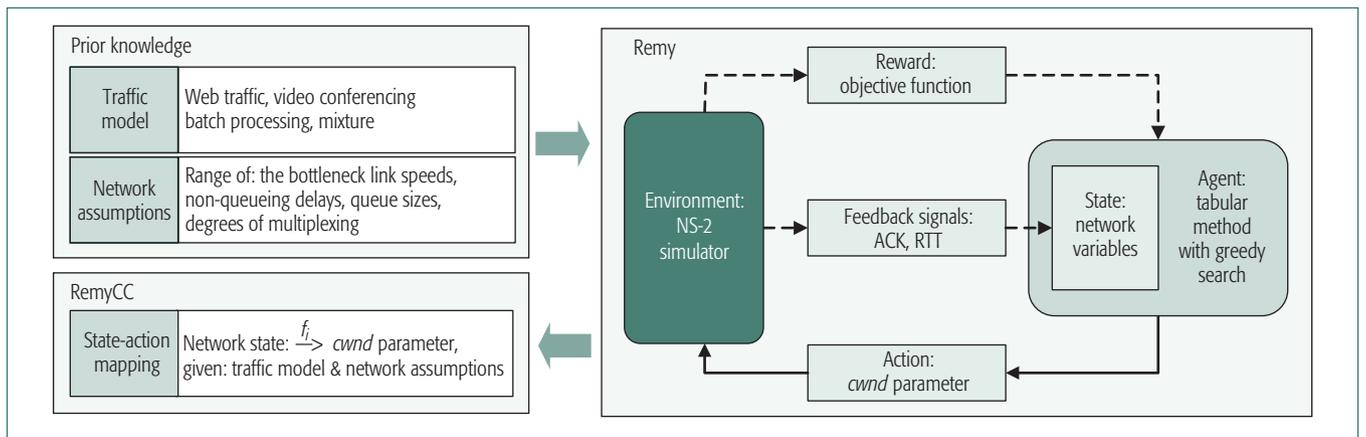
FIGURE 2. Remy's mechanism illustration [3].
