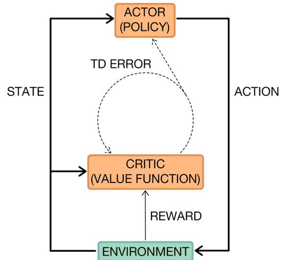
Fig. 4. Actor-critic set-up. The actor (policy) receives a state from the environment and chooses an action to perform. At the same time, the critic (value function) receives the state and reward resulting from the previous interaction. The critic uses the TD error calculated from this information to update itself and the actor. Recreated from [135].
