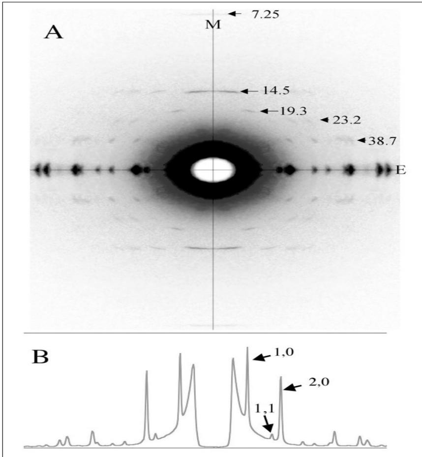
We are looking at projection of hexagonal lattice onto a plane. Insect muscle is highly ordered so you get lots of sharp spots along the equator. Note that they vary in intensity
