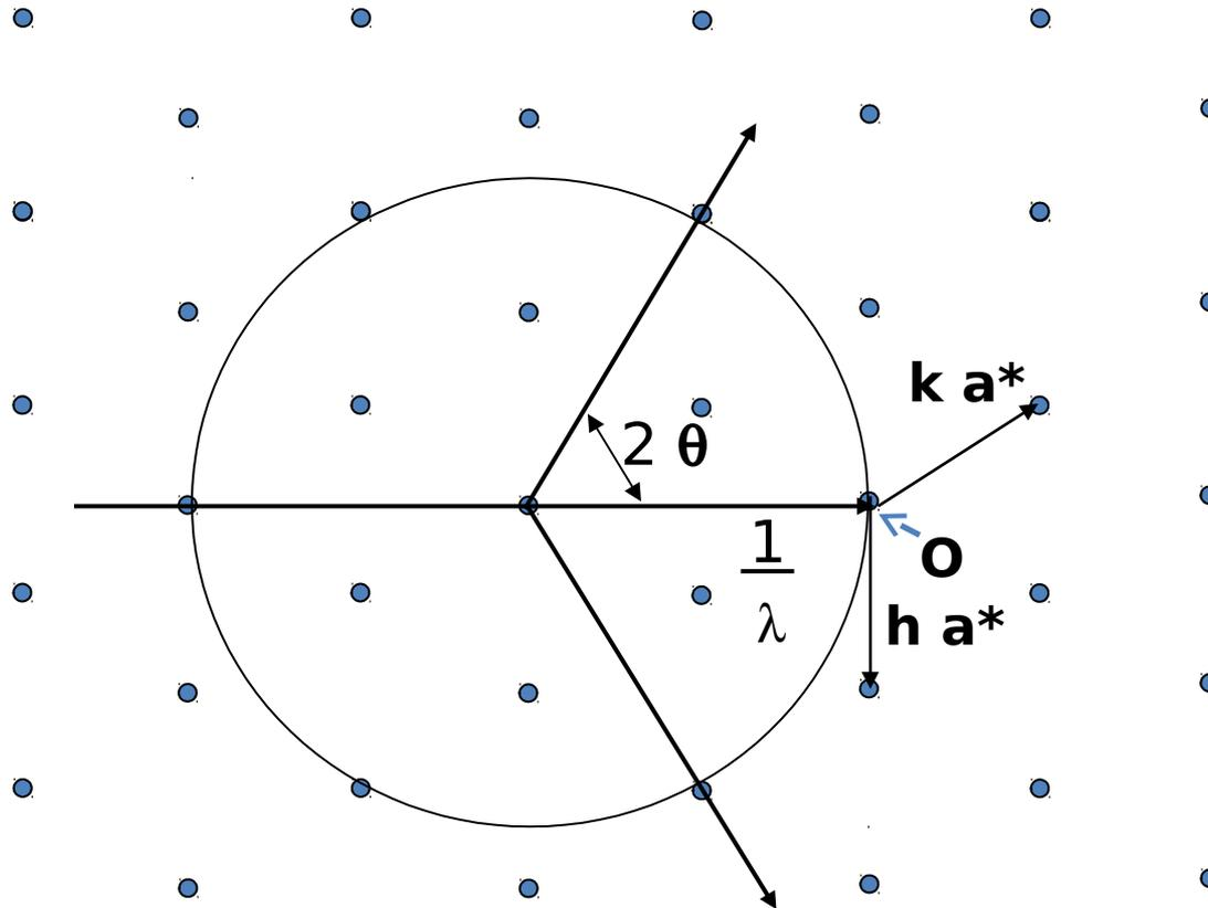
For every lattice in real space there is a corresponding lattice in “reciprocal” i.e. diffraction space. Distances between lattice points are proportional to  $1/\text{lattice dimensions}$  in real space. The origin of the reciprocal lattice is at  $O$ . Lattice points (corresponding to diffraction spots one can observe) are indexed by Miller indices  $h$  and  $k$
