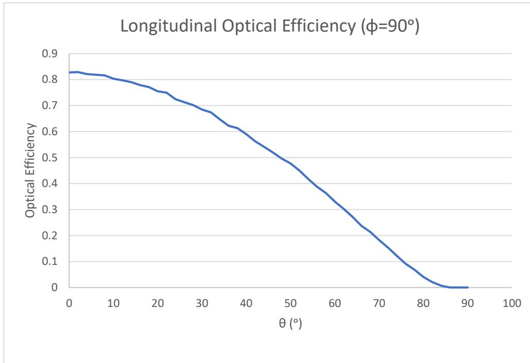
Fig. 17. Optical efficiency depending on the incidence angle in the longitudinal plane.
