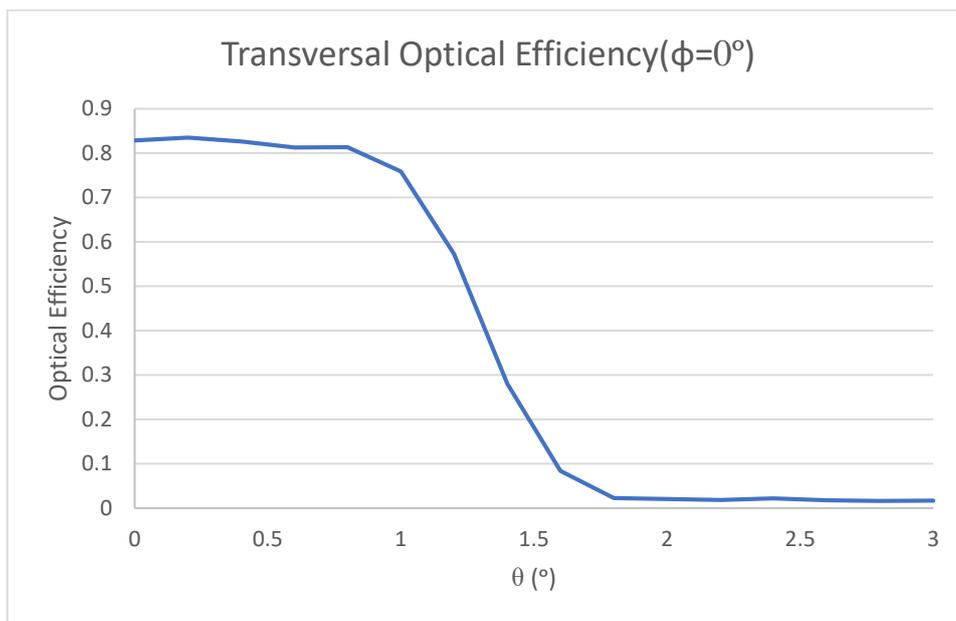
Fig. 18. Transversal efficiency curve of the collector.
