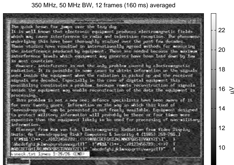
Figure 17.2: RF signal from a Toshiba laptop reconstructed several rooms away, through three plasterboard walls (courtesy of Markus Kuhn [752]).
