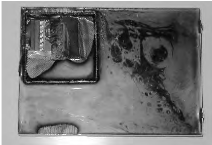
Figure 16.2: The 4758 partially opened showing (from top left downward) the circuitry, aluminium electromagnetic shielding, tamper sensing mesh and potting material (courtesy of Frank Stajano)
