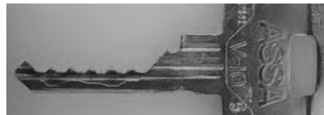
Figure 11.3: Bump key for a sidebar lock
