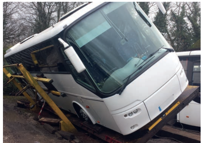
▲ Figure 1.5.32b A coach being tilted to test its stability
