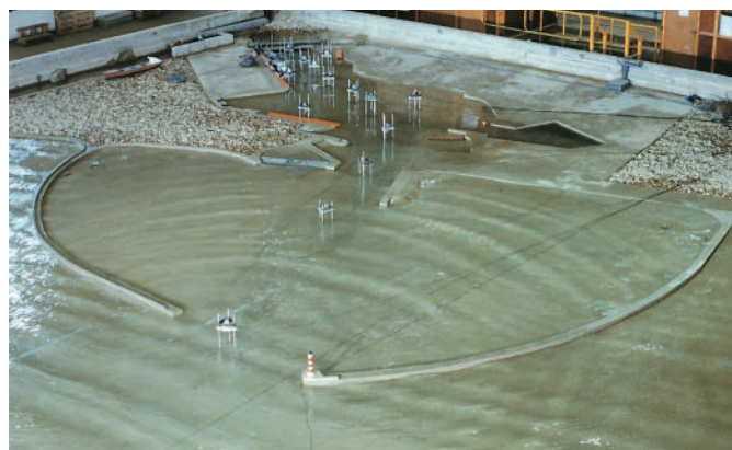
▲ Figure 3.1.11 Model of a harbour used to study wave behaviour
