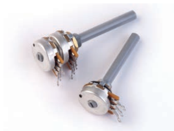
▲ Figure 4.2.24c Variable resistor (potentiometer)
