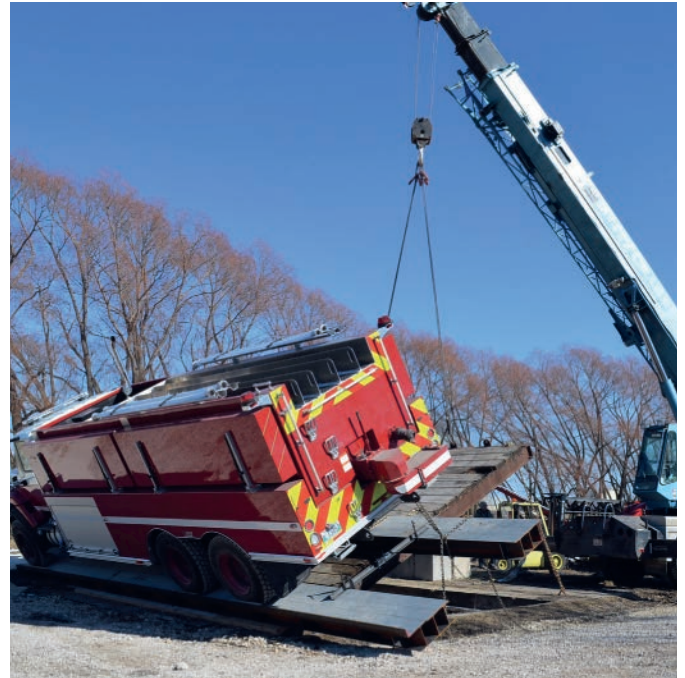
▲ Figure 1.5.32a A fire truck under test to find its centre of gravity
