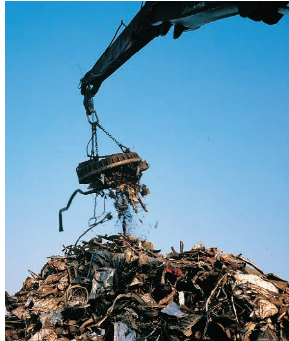
▲ Figure 4.1.12 Electromagnet being used to lift scrap metal
