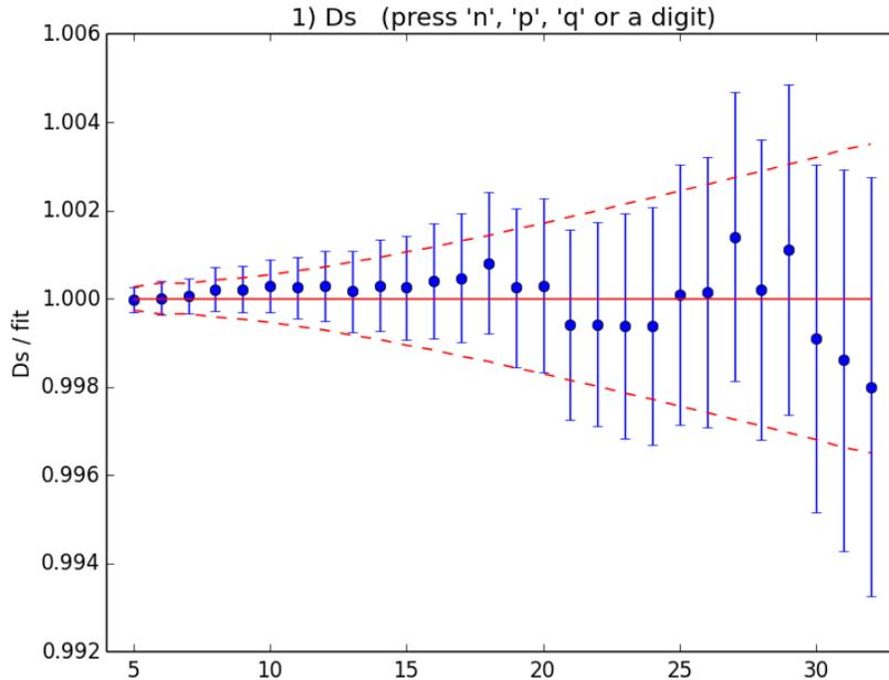
The points with error bars are the correlator data points; the fit result is 1.0 in this plot, of course, and the dashed lines show the uncertainty in the fit function evaluated with the best-fit parameters. Fit and data agree to within errors. Note how the fit-function errors (the dashed lines) track the data errors. In general the fit function is at least as accurate as the data. It can be much more accurate, for example, when the data errors grow rapidly with  $t$ .
