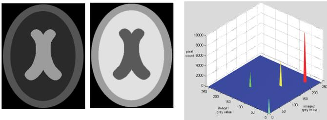
The maxima of a mutual histogram of two images, can be used to convert the region gray level representation in one image into the representation of the other image.
