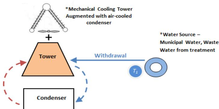
**Withdrawal:** Report the cooling tower makeup water that is removed from a water body.
