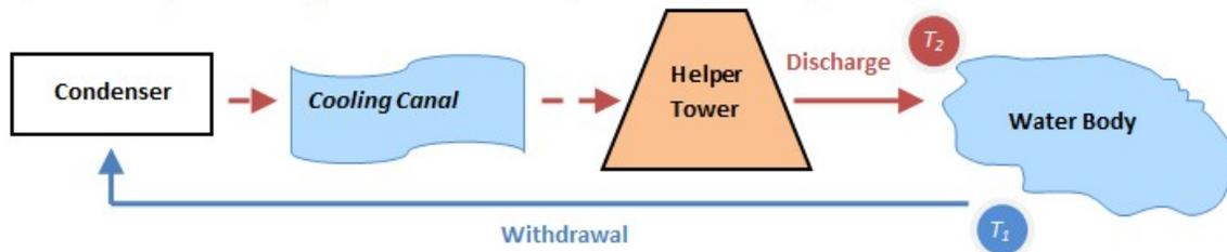
\* Helper Tower can be positioned before, after or along the canal.
