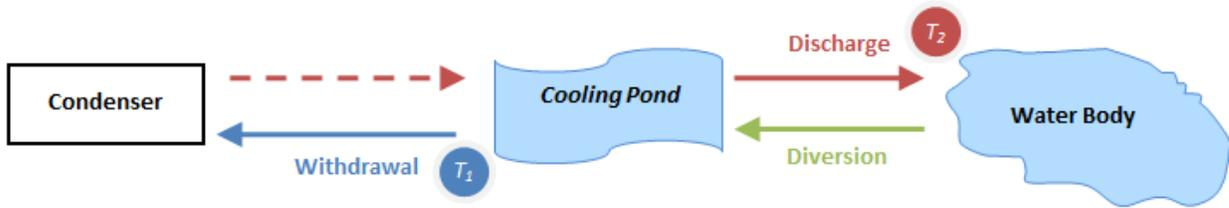
**Withdrawal:** Report the water flow to the condenser from the cooling pond.
