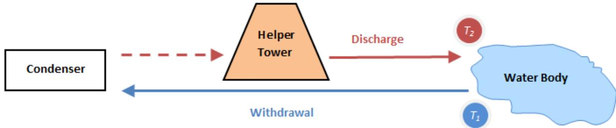
**Withdrawal:** Report the water that is removed from a water body for cooling, i.e. water used through the condenser.
