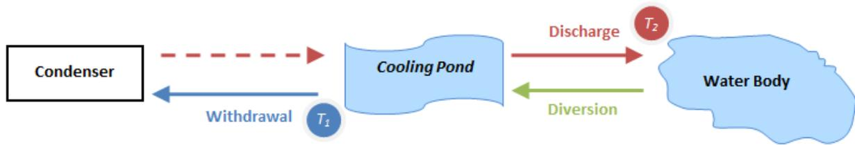
**Withdrawal:** Report the water flow to the condenser from the cooling pond.
