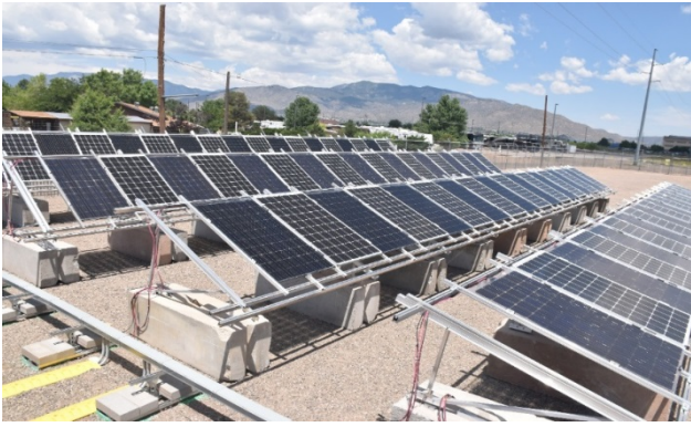
Fig. 5. Bifacial PV module test bed at Sandia. Four rows of PV modules with tilt angles from 15° to 45°. Backside irradiance measured for top and bottom of PV module near the center of each row. Front side irradiances are also measured.
