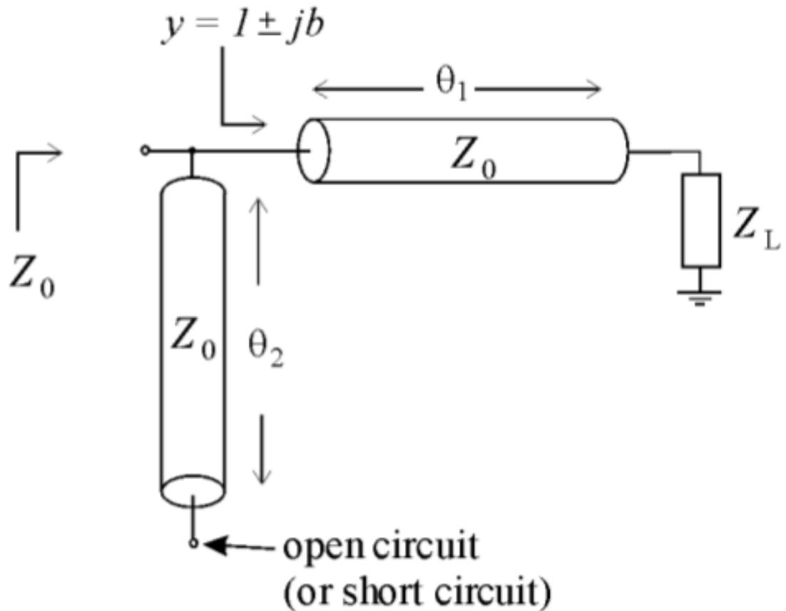
A single stub matching network can be designed to produce maximum power transfer to the load, at a single frequency. The matching network has two design parameters:
