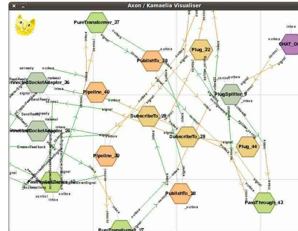
Clearly at this point we've reached the limits of the visualiser. Viewing the network of components as a flat layout is useful from the perspective of seeing "what's going wrong, if anything" for small systems, but for large ones, wrapping up the structure would be nicer. This is something that would be great for someone to work one, but we've not had the time for this.
