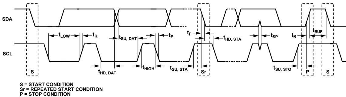
Figure 3. I<sup>2</sup>C Interface Timing Diagram
