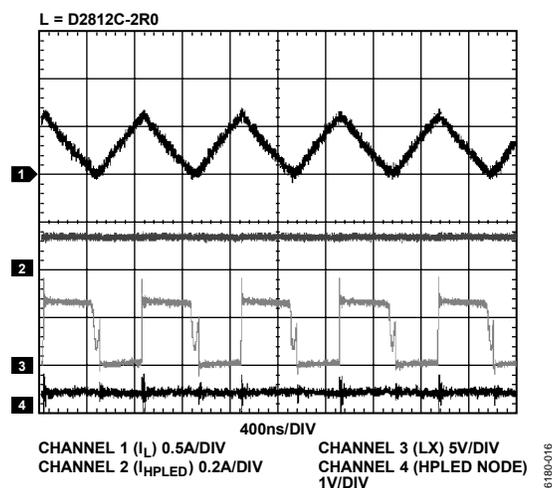
Figure 10. Inductor Current, Two LEDs Torch Mode, LED Current = 130 mA, V<sub>DD</sub> = 3.6 V
