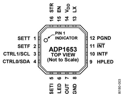
Figure 4. Pin Configuration
