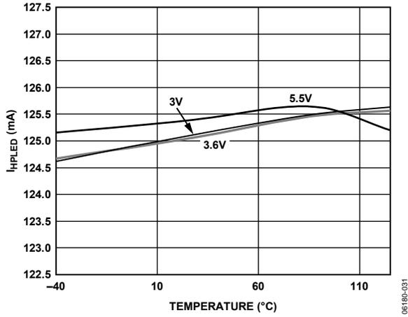
Figure 23. HPLED Regulation, Set at 125 mA, HPLED Register = 00110 (Binary), SETF = V<sub>DD</sub>
