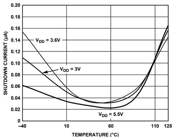
Figure 19. Shutdown Current vs. Temperature, EN = 0 V
