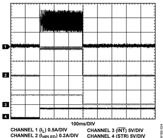
Figure 17. Flash Untimed Mode, Two LEDs, Timer = 300 ms, I<sub>HLED</sub> = 380 mA, V<sub>DD</sub> = 3.6 V
