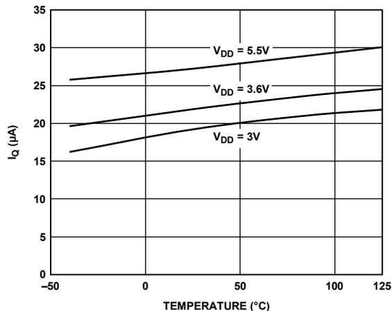
Figure 20. Quiescent Current vs. Temperature, EN = V<sub>DD</sub>, LED Functions Disabled
