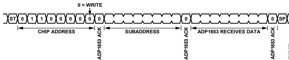
Figure 26. I<sup>2</sup>C Write Sequence
