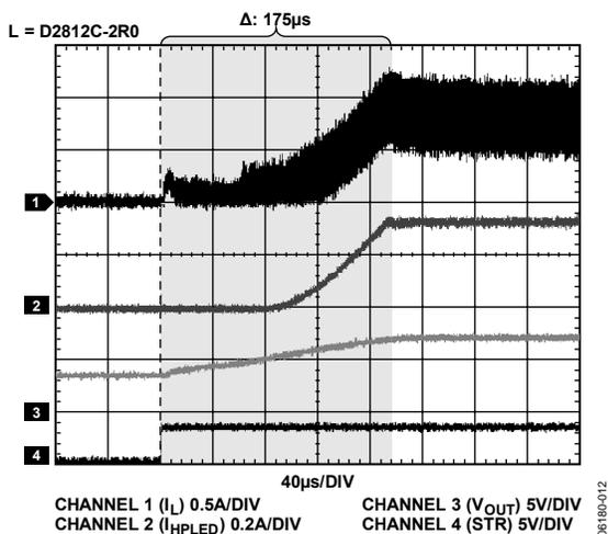
Figure 6. Startup, Two LEDs Flash Mode, LED Current = 335 mA, V<sub>DD</sub> = 3.6 V
