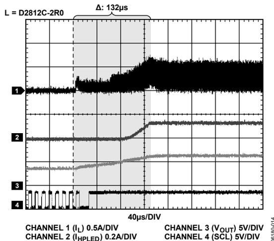
Figure 8. Startup, Two LEDs Torch Mode, LED Current = 130 mA, V<sub>DD</sub> = 3.6 V
