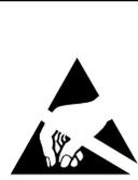
**ESD (electrostatic discharge) sensitive device.** Charged devices and circuit boards can discharge without detection. Although this product features patented or proprietary protection circuitry, damage may occur on devices subjected to high energy ESD. Therefore, proper ESD precautions should be taken to avoid performance degradation or loss of functionality.
