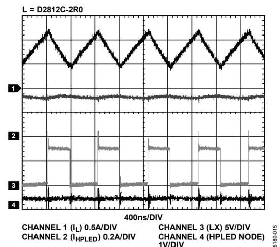
Figure 9. Inductor Current, Two LEDs Flash Mode, LED Current = 335 mA, V<sub>DD</sub> = 3.6 V
