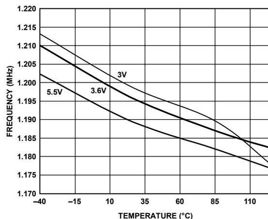
Figure 22. Oscillator Frequency vs. Temperature vs. V<sub>DD</sub>
