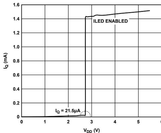
Figure 21. Quiescent Current vs. V<sub>DD</sub>, V<sub>DD</sub> Swept from 5.5 V to 0 V, ILED Active at 2.5 mA Until UVLO Threshold
