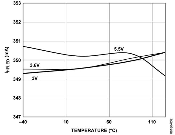
Figure 24. HPLED Regulation, Set at 350 mA, HPLED Register = 10101 (Binary), SETF = V<sub>DD</sub>
