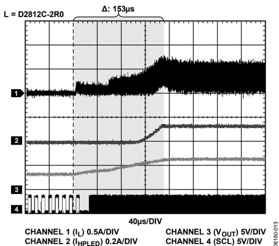
Figure 7. Startup, Two LEDs Torch Mode, LED Current = 130 mA, V<sub>DD</sub> = 3.2 V
