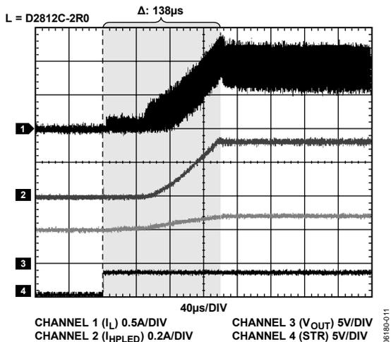
Figure 5. Startup, Two LEDs Flash Mode, LED Current = 335 mA, V<sub>DD</sub> = 3.2 V
