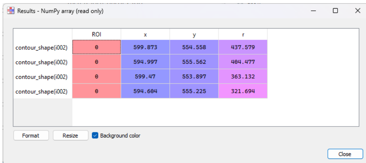
Fig. 58: Select the “Contour detection” tool in the “Computing” menu, with the same parameters as before (shape “Circle”). On this image, there are two fringes, so four circles are fitted. The “Results” dialog opens, and displays the fitted circle parameters. Click “OK”.
