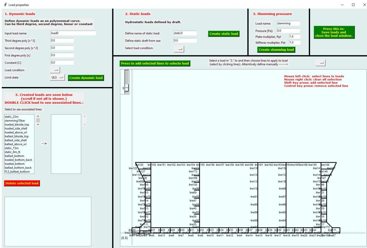
Slamming loads can be specified separately. The multiply factors are the slamming pressure to be used on plate and stiffener respectively. For example for a 10 bar pressure:
