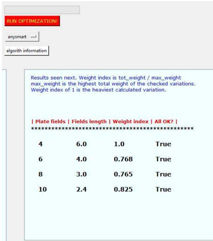
In this case 8 plate fields with length of 3 meters will give the lowest weight. 6 plate fields are almost equal.
