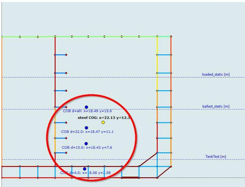
Development of weight and COG is recorded each time the structure changes. The resulting plot can be seen by pressing the “weights” button.
