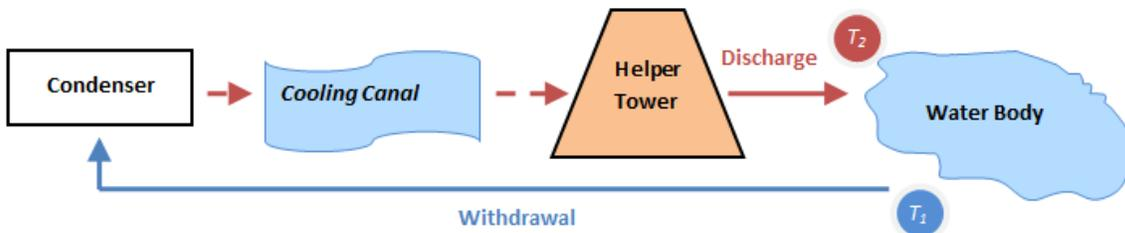
\* Helper Tower can be positioned before, after or along the canal.
