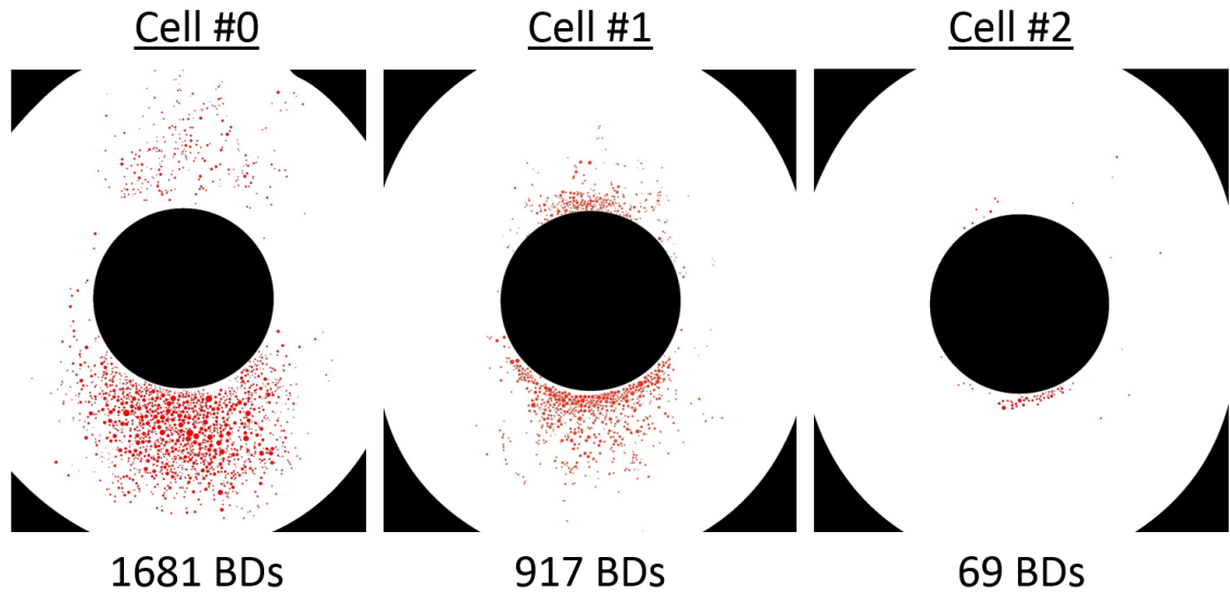
Figure 33: CLIC Crab cavity crater distribution from post-mortem analysis of the the first three RF input side cell walls [51]. The abruptly decaying number of craters is consistent with Fig. 31 and 32.
