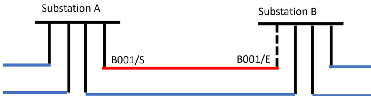
Diagram illustrating the calculation used in the first stage single end feeding arrangement calculating single end feeding load of B001/S at Substation A when there is an outage at Substation B connected to B001/E.
