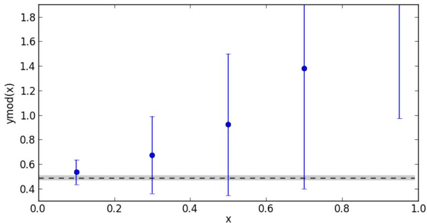
The constant is consistent with all of the data in `ymod[i]`, even at `x[i]=0.95`, because `ymod[i]` has much larger errors for larger `x[i]` because of the correction terms.
