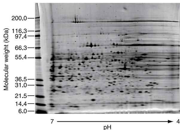
**Figure 2.** SYPRO® Ruby protein gel stain on a 2-D gel. Rat liver lysate (20 µg) separated on a pH 4–7 IPG strip and then on a NuPAGE® 4–12% Bis-Tris gel and stained with SYPRO® Ruby gel stain following the rapid stain protocol.
