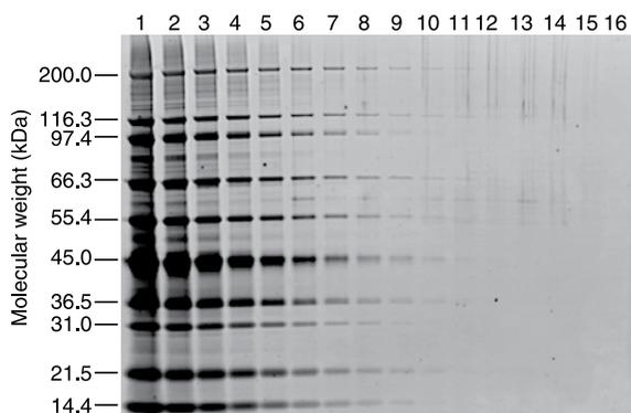
**Figure 1.** SYPRO® Ruby protein gel stain on a 1-D gel. Two-fold dilution series of Mark12™ unstained standards supplemented with ovalbumin, separated on a NuPAGE® 4–12% Bis-Tris gel, and stained with SYPRO® Ruby gel stain following the rapid stain protocol. Lane 9 is approximately 1 ng protein.
